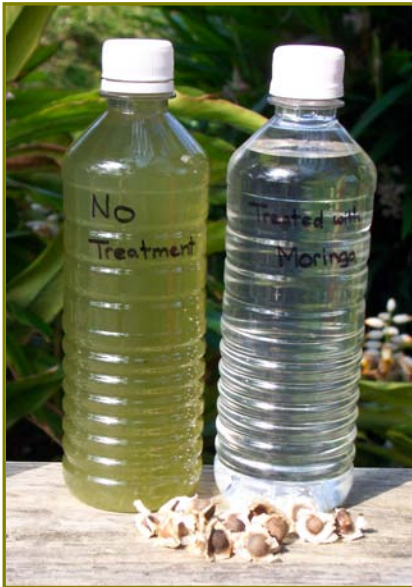
Contaminated water before and after Moringa treatment Photo by Beth Doerr
